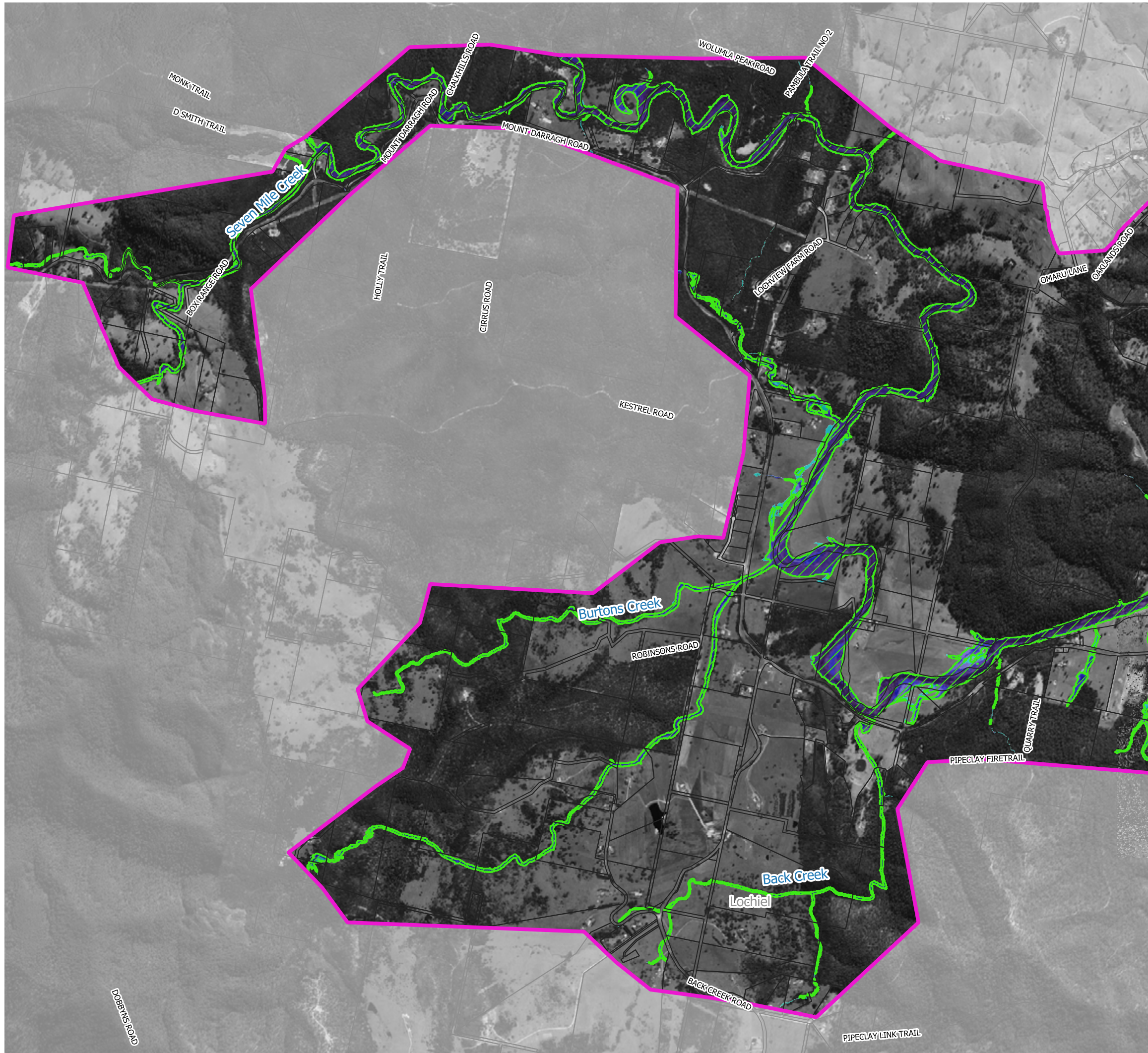
Figure 55.1 Peak 1% AEP Water Depths with 41% Rainfall Increases
