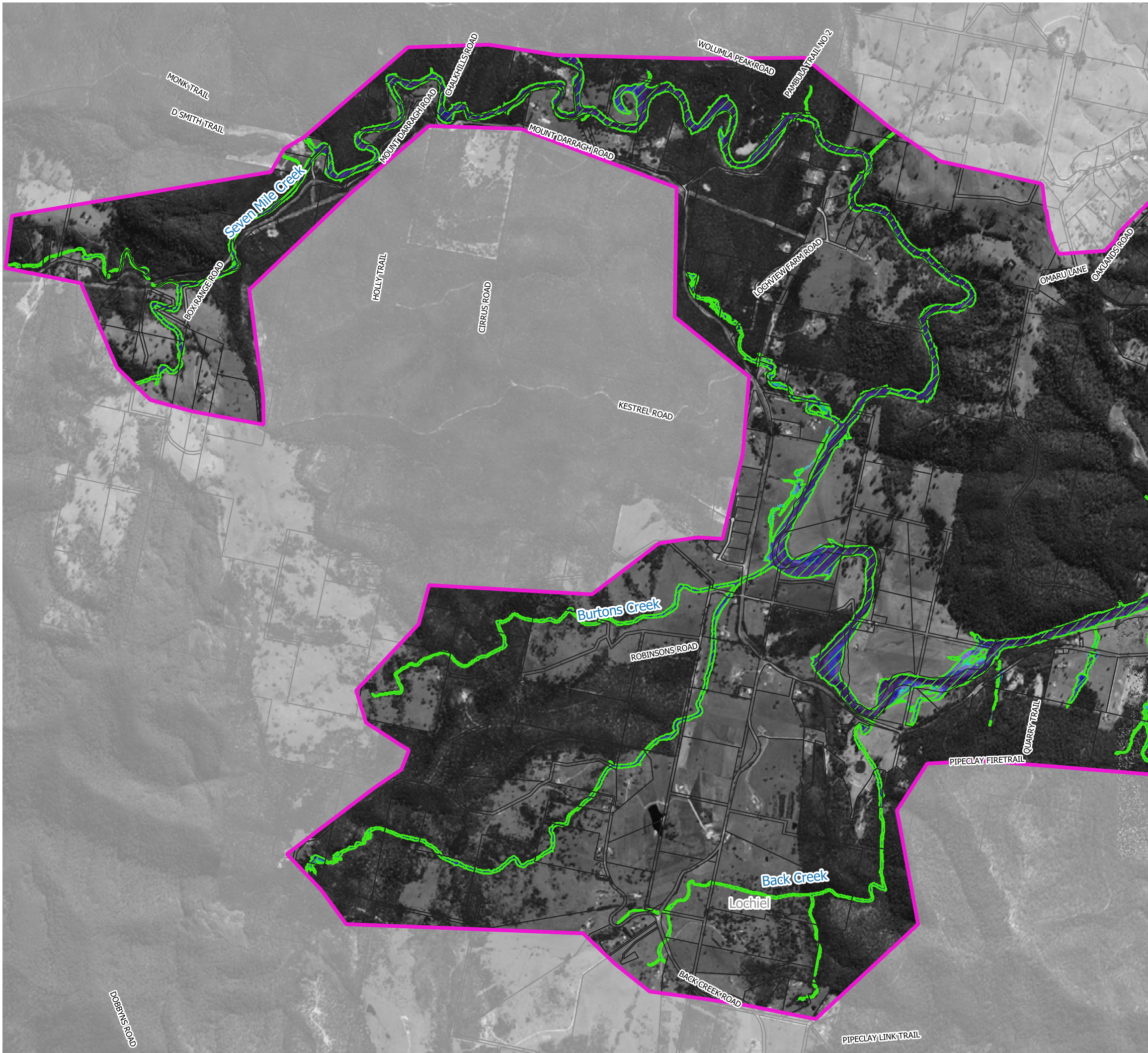
Figure 56.1 Peak 1% AEP Water Depths with 18% Rainfall Increases and 0.4m Sea Level Rise
