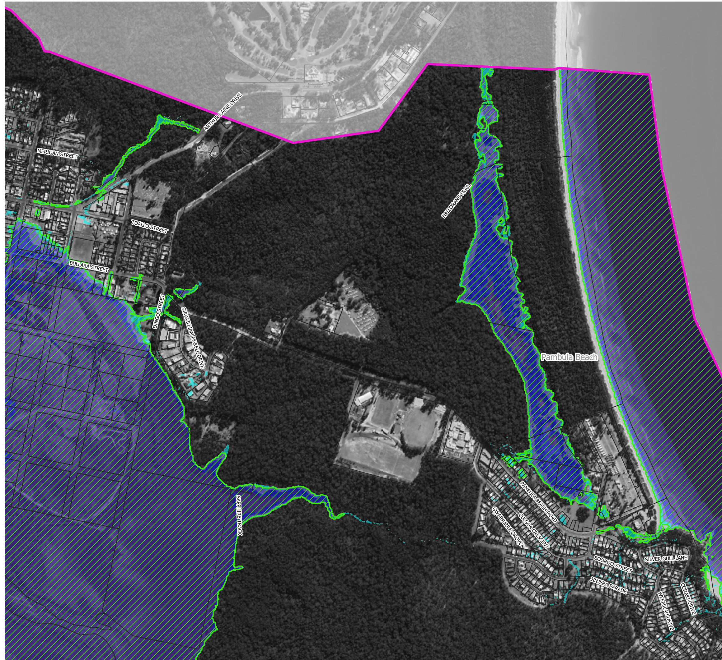
Figure 55.6 Peak 1% AEP Water Depths with 41% Rainfall Increases
