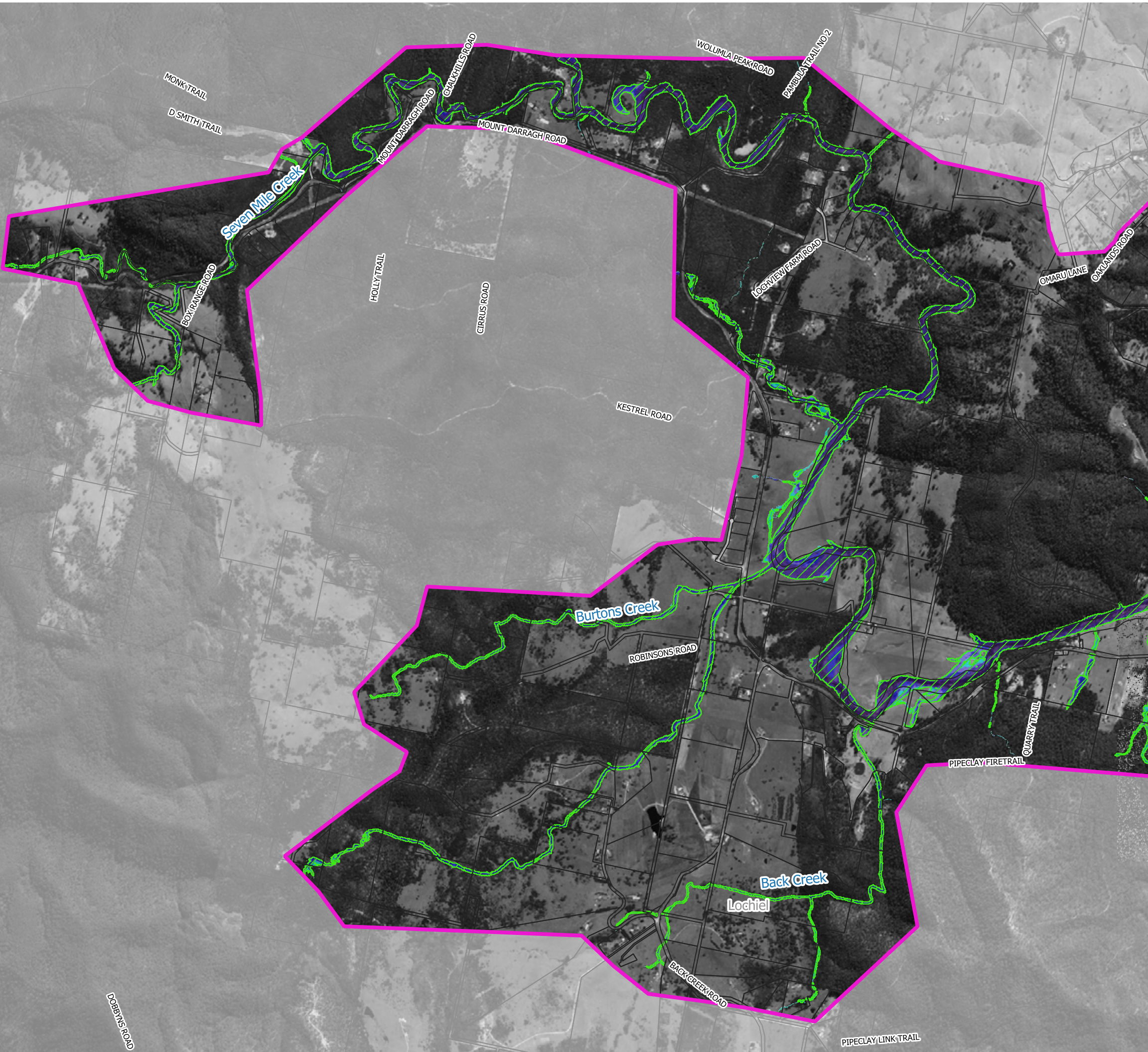
Figure 54.1 Peak 1% AEP Water Depths with 18% Rainfall Increases
