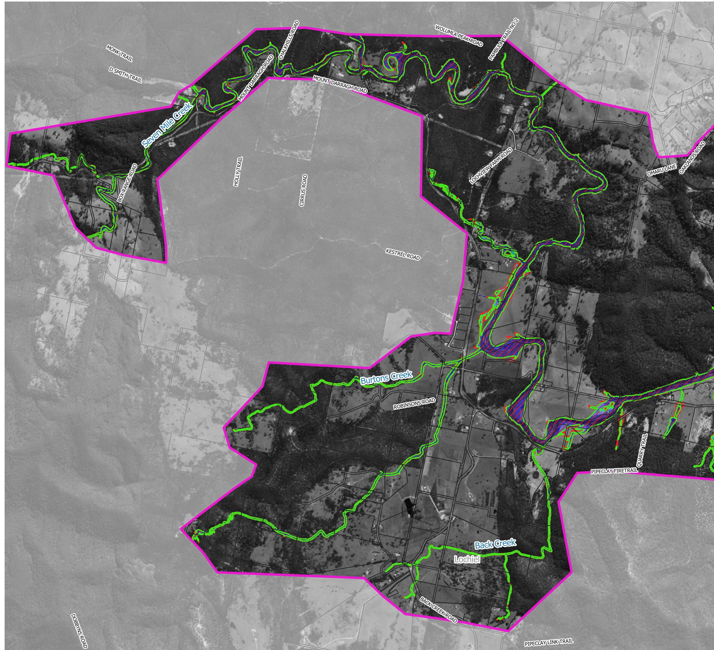
Figure 59.1 Peak 1% AEP Water Depths with 41% Rainfall Increases and 0.9m Sea Level Rise and 0.9m Increase in River Entrance Elevation
