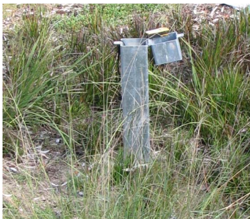
Figure 2-3: Existing bore PPK1 showing typical bore capping
