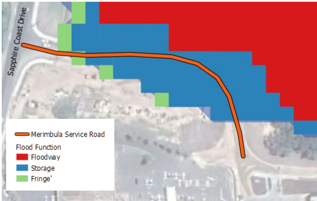
Figure 8-3 Merimbula Service Road Location and Flood Function
