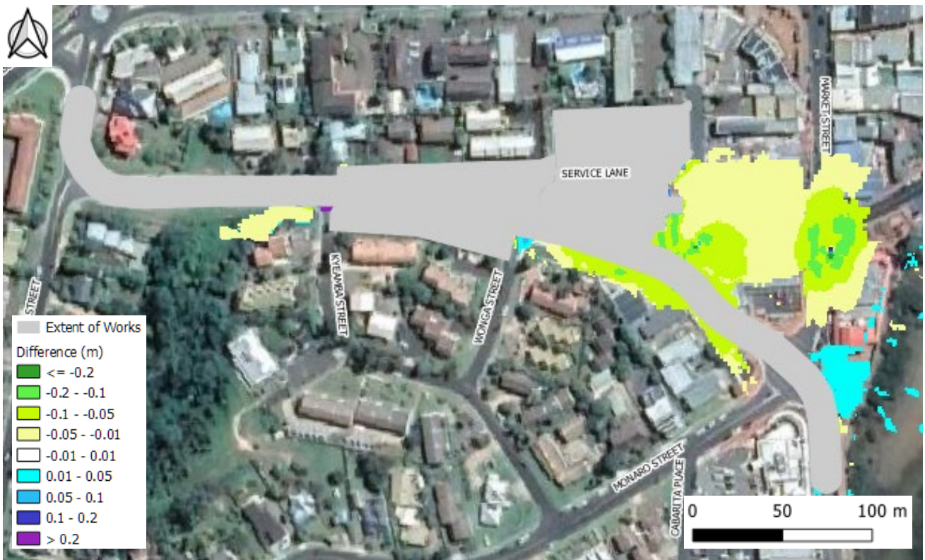
Figure 8-5 5% AEP Bypass Impacts
