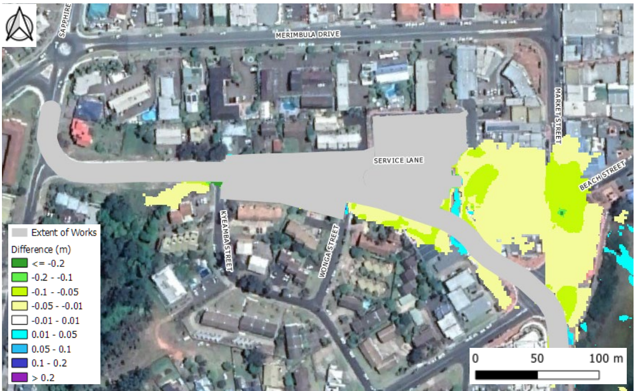
Figure 8-6 1% AEP Bypass Impacts
