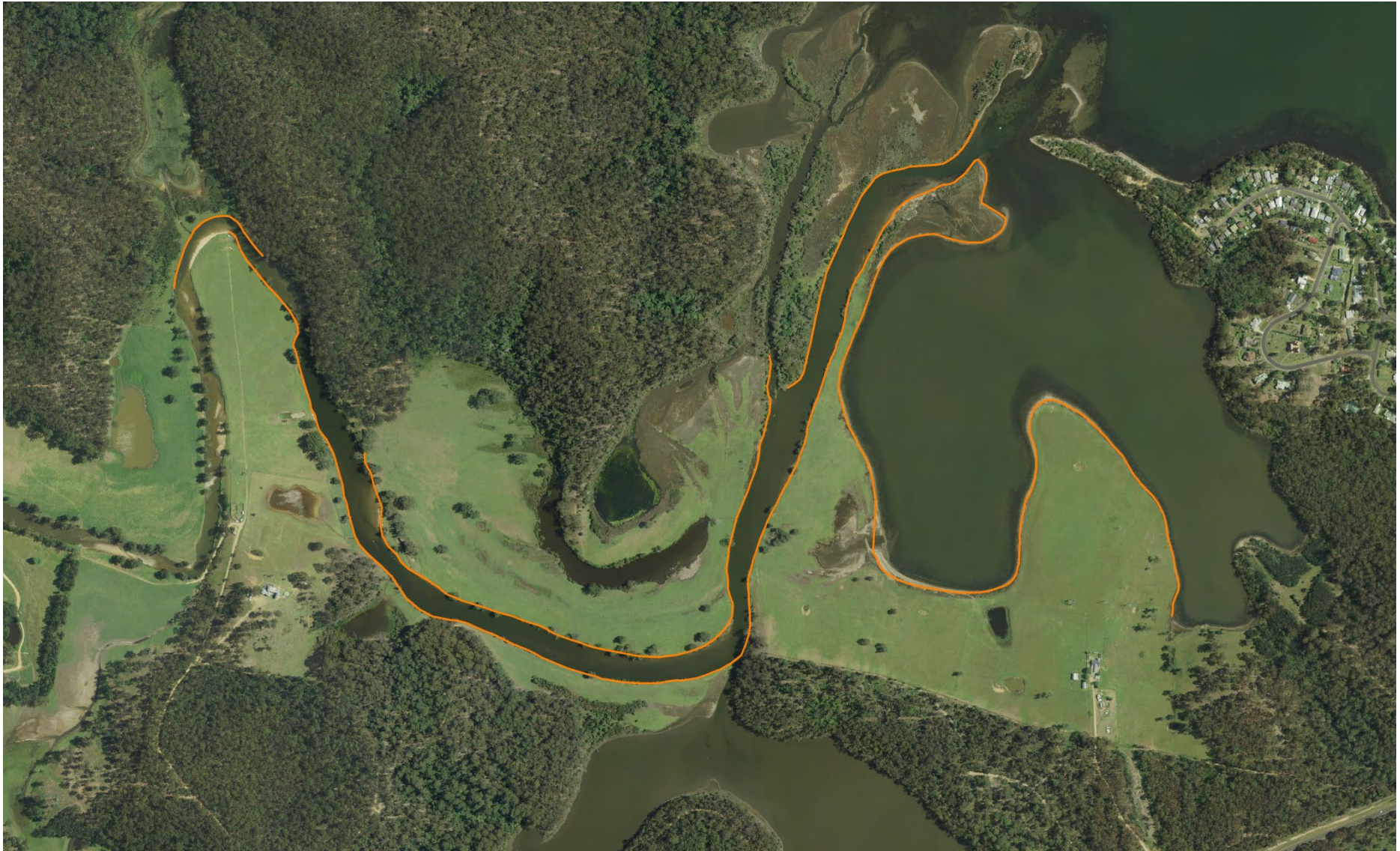
Figure 2: Zones of Bank Erosion/Slumping, Narira Creek Estuary Branch
