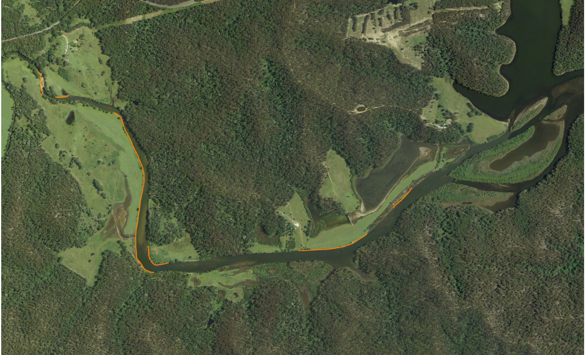
Figure 1: Zones of Bank Erosion/Slumping, Dignams Creek Estuary Branch
