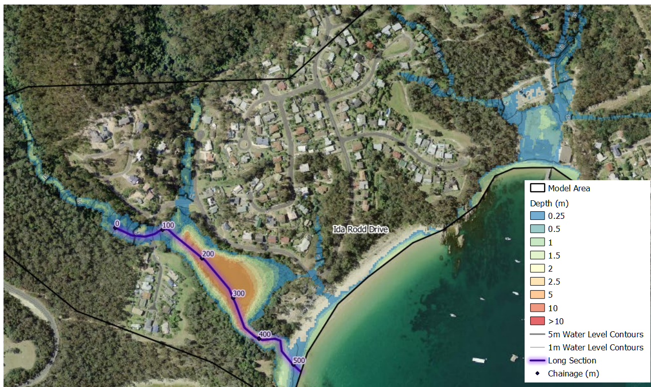
Figure 6-16 Lake Cocora 1% AEP Flooding & Long Section Chainage
