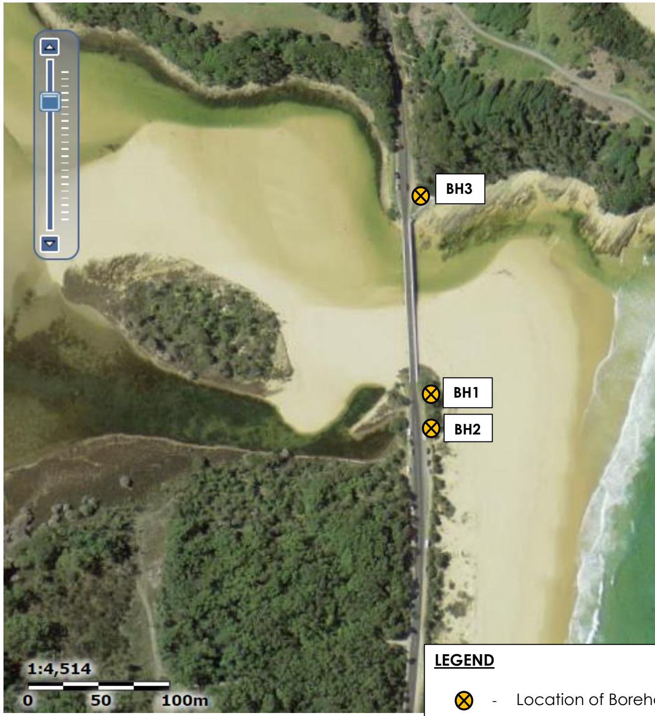
BEGA VALLEY SHIRE COUNCIL PROPOSED CUTTAGEE BRIDGE AERIAL PHOTOGRAPH & LOCATIONS OF BOREHOLES
