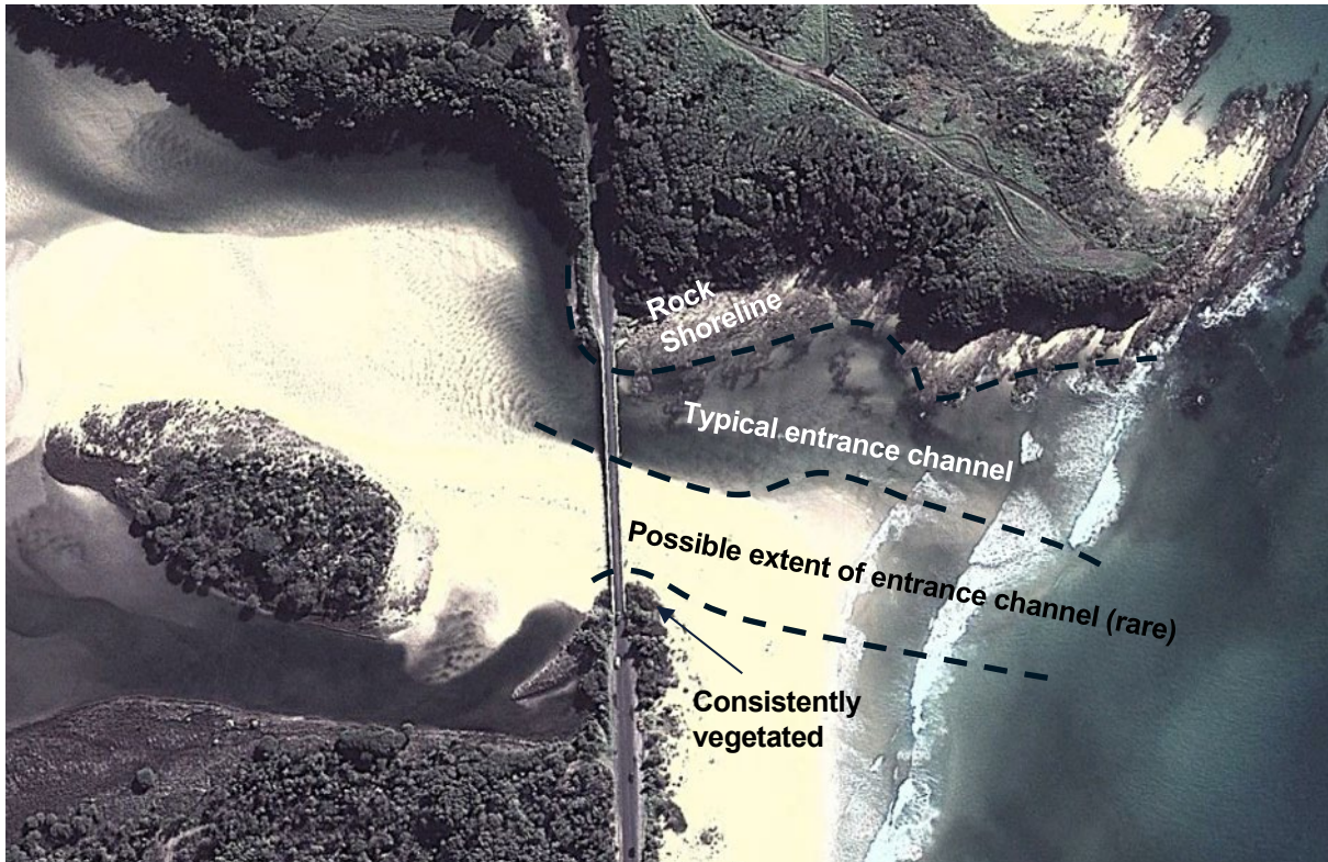
Figure 1: Summary of Cuttagee Lake Entrance Conditions
