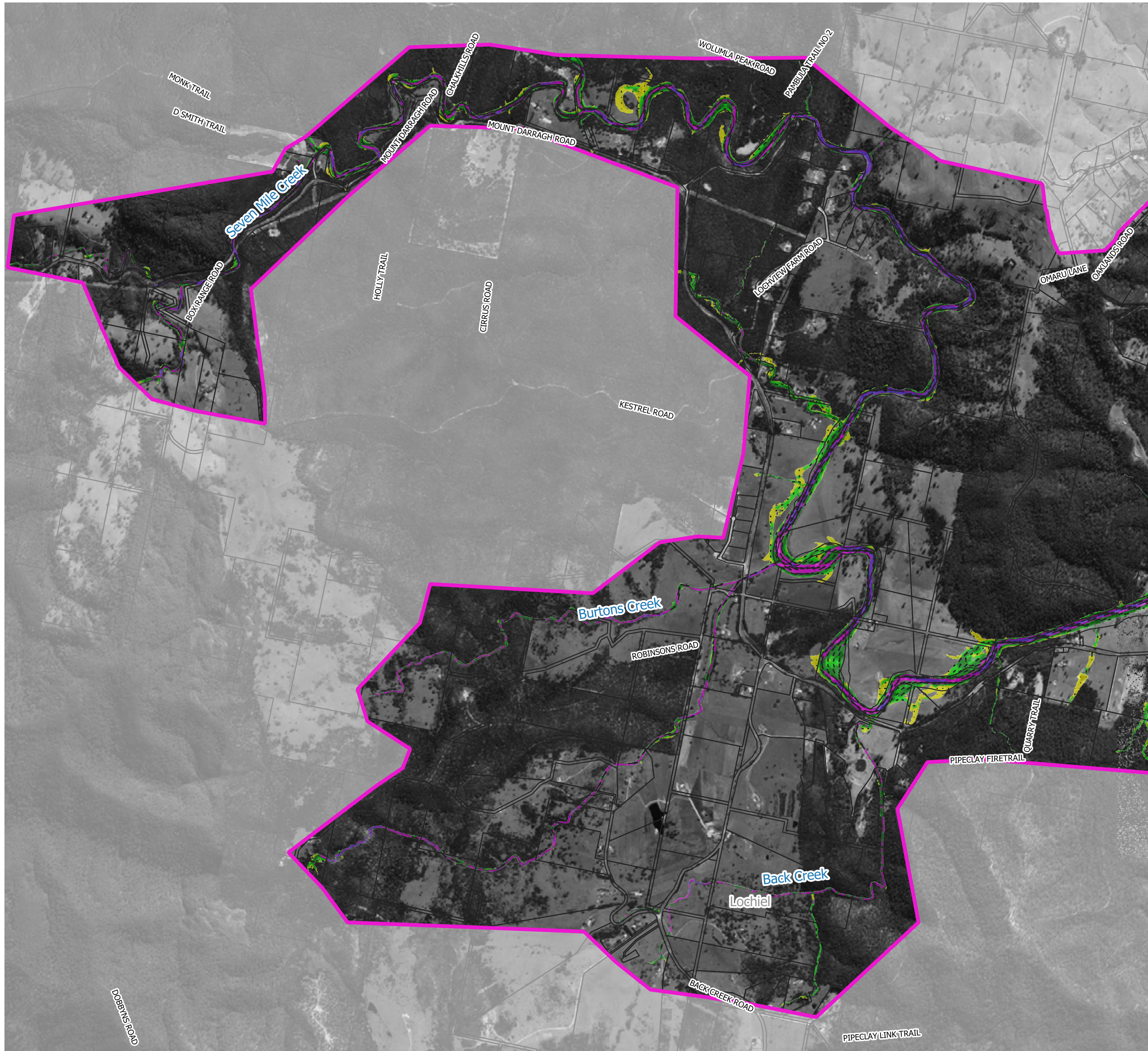
Figure 31.1 Peak Floodwater Speed for the 0.2% AEP Flood
