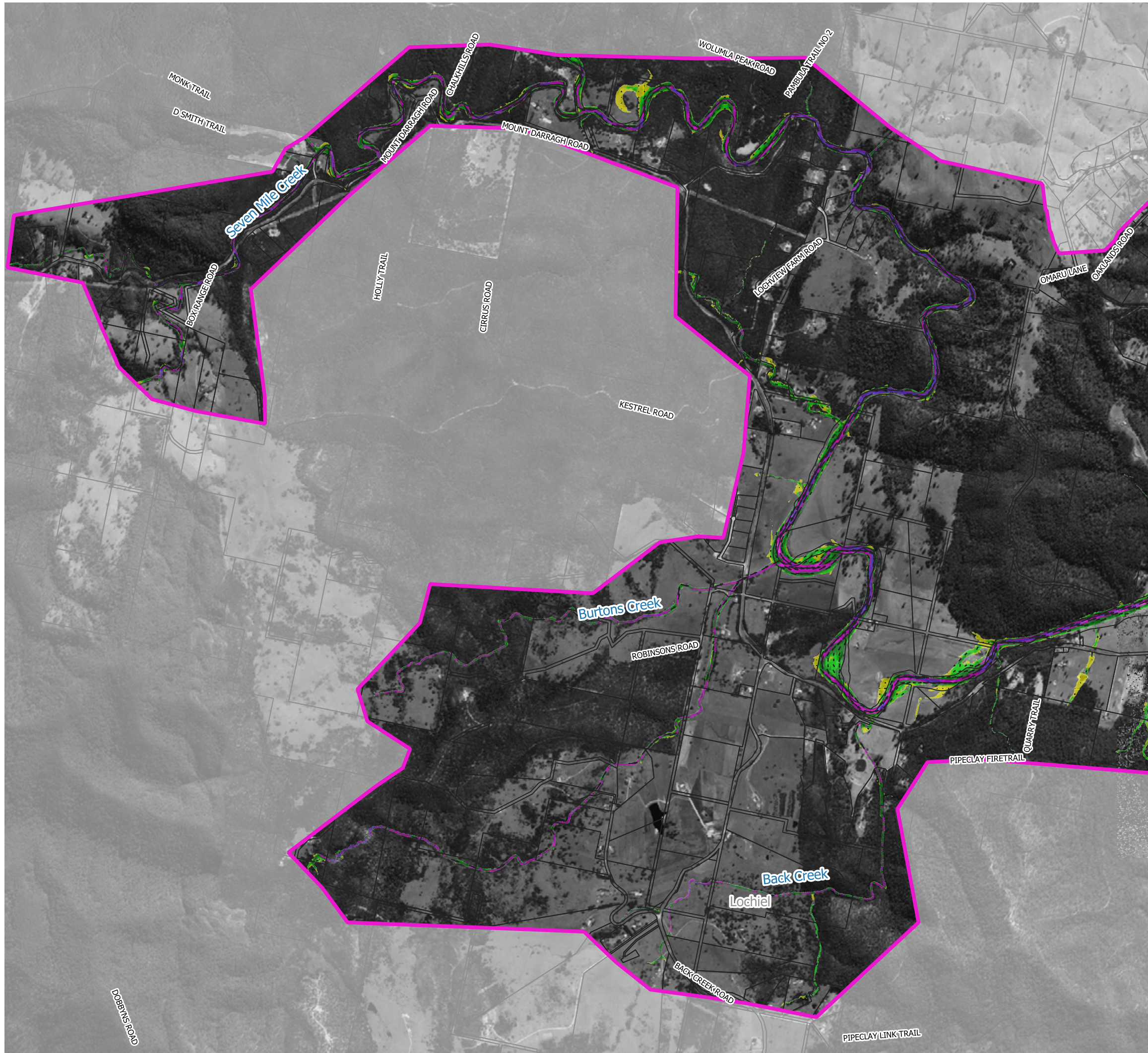
Figure 28.1 Peak Floodwater Speed for the 2% AEP Flood
