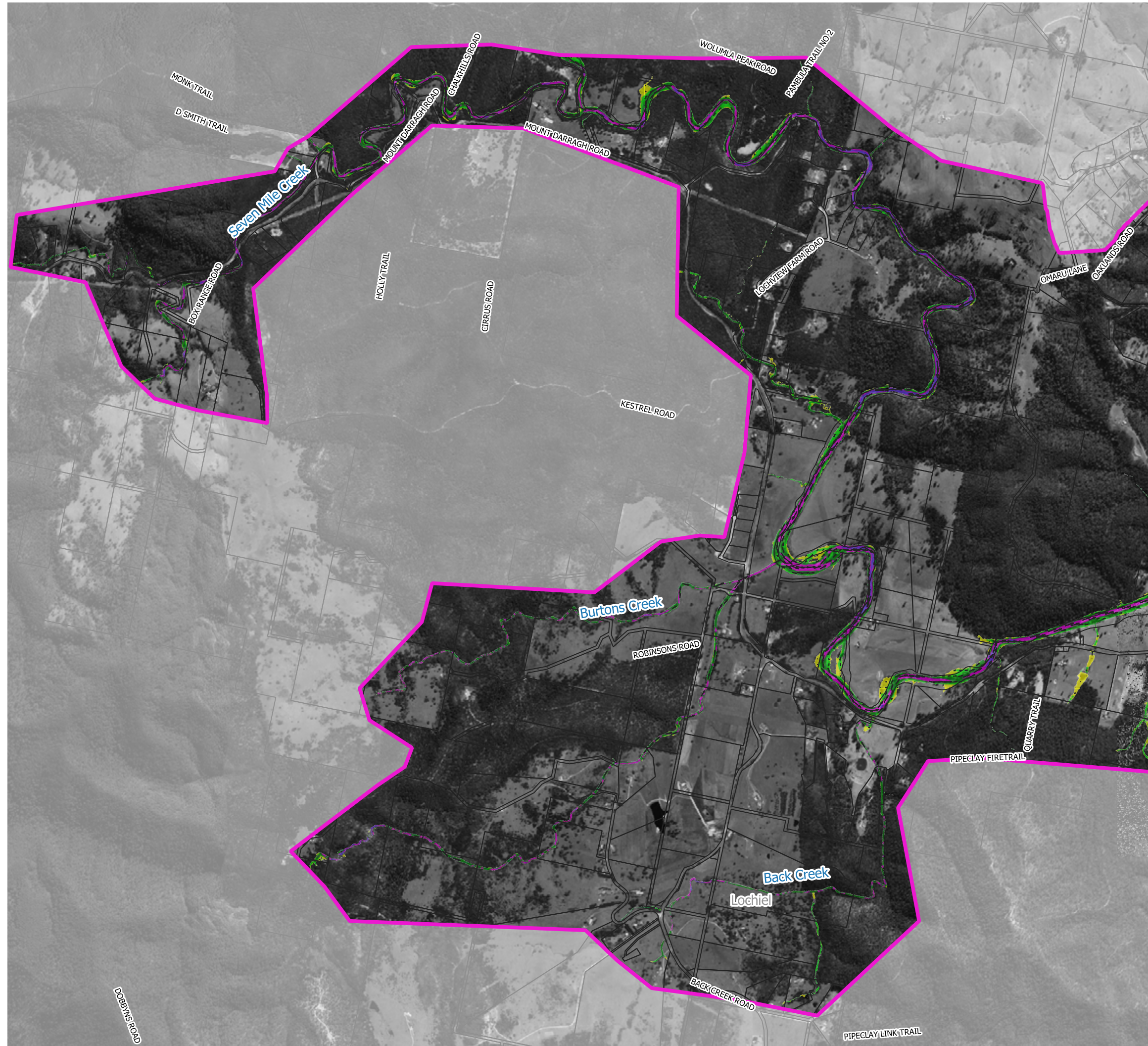
Figure 26.1 Peak Floodwater Speed for the 10% AEP Flood
