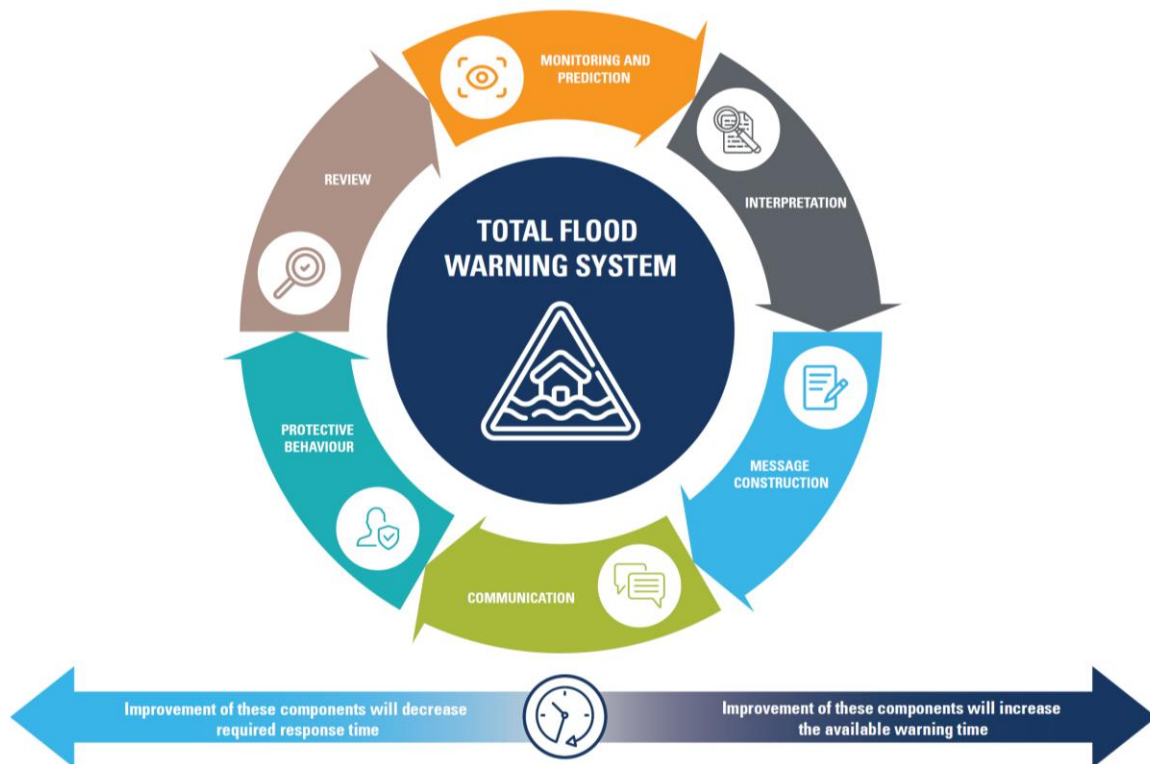
Figure C.1 The components of the Total Flood Warning System (Australian Emergency Manual Series, Manual 21, Flood Warning, Australian Government 2009)
