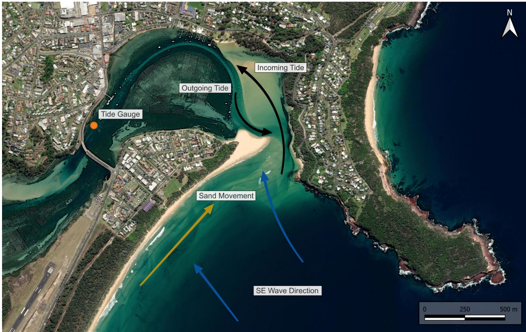
Figure 8 Merimbula Lake entrance bar sediment transport conceptual model
