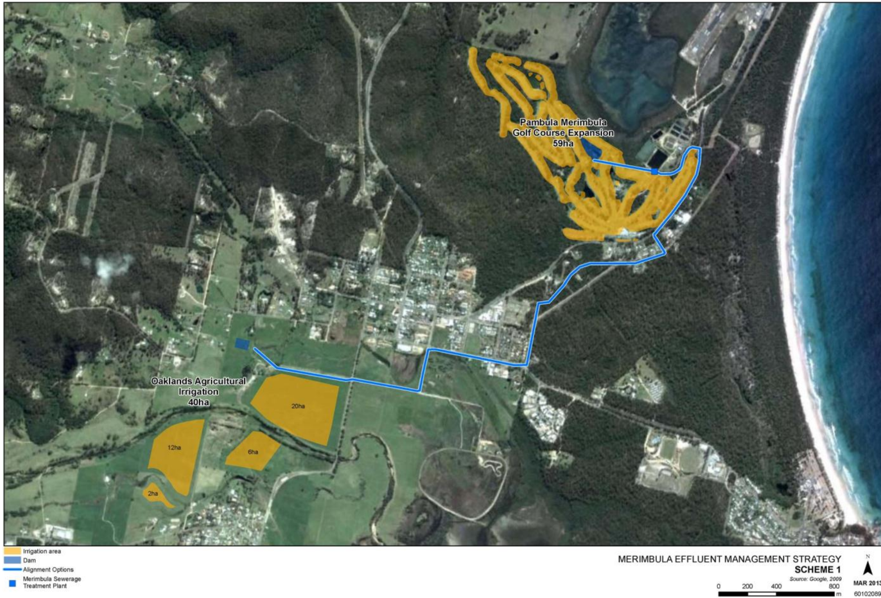
Figure 2 Effluent Reuse Scheme 1 Plan View
