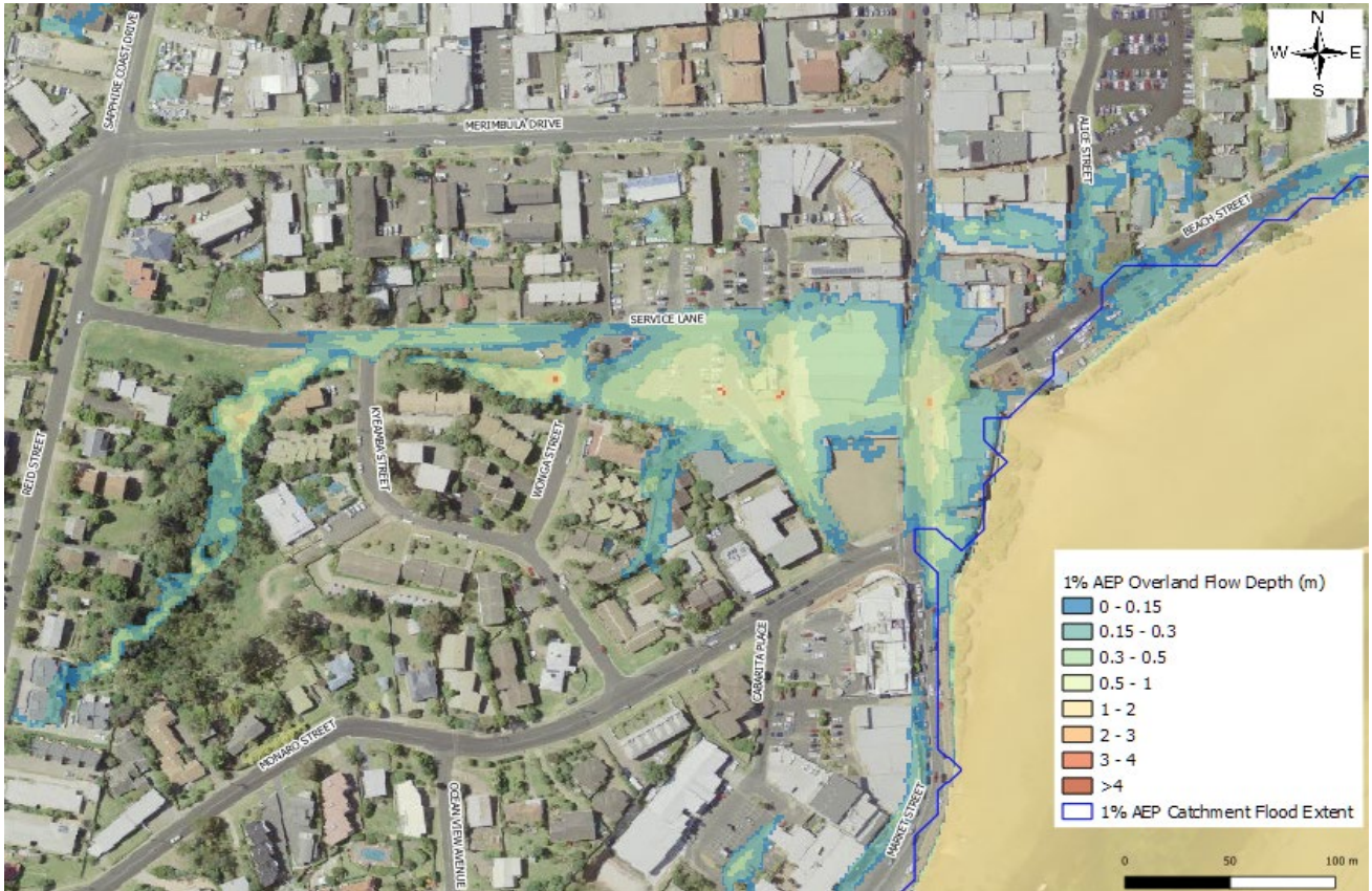
Figure 3-1 Overflow Flooding in the Merimbula CBD
