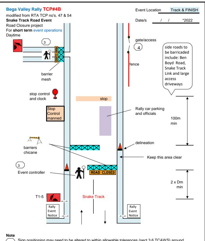
Sign positioning may need to be altered to within allowable tolerences (sect 3.6 TCAWS) around local obstructions. Minimum requirements to be noted on TCP
