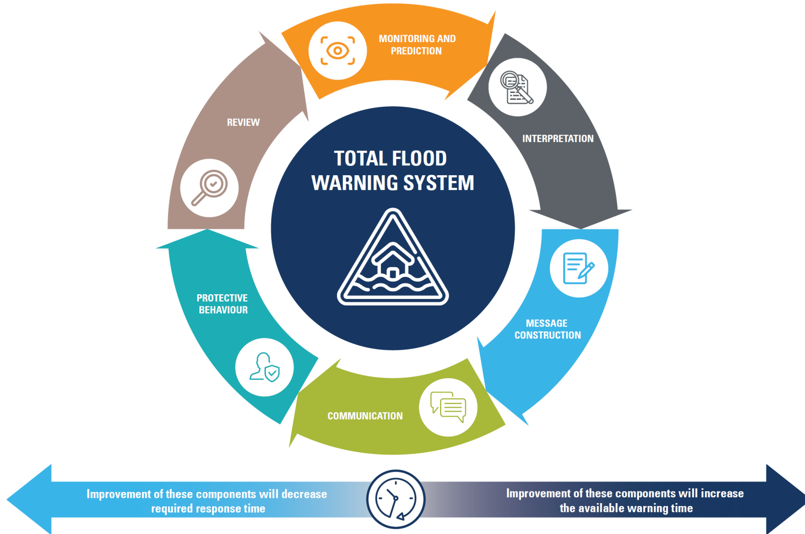
Figure 1-1 The components of the Total Flood Warning System (Australian Emergency Manual Series, Manual 21, Flood Warning, Australian Government 2009)
