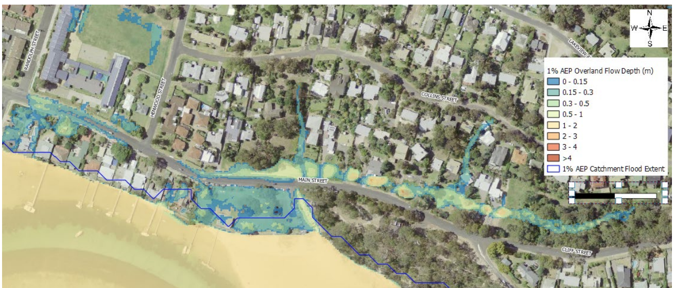
Figure 2-2 Overland Flooding in Main Street
