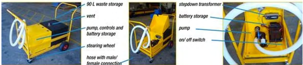
Photo H: Images of the mobile sewage pump out trolley ('Muck Truck') as supplied by Superior Jetties.
