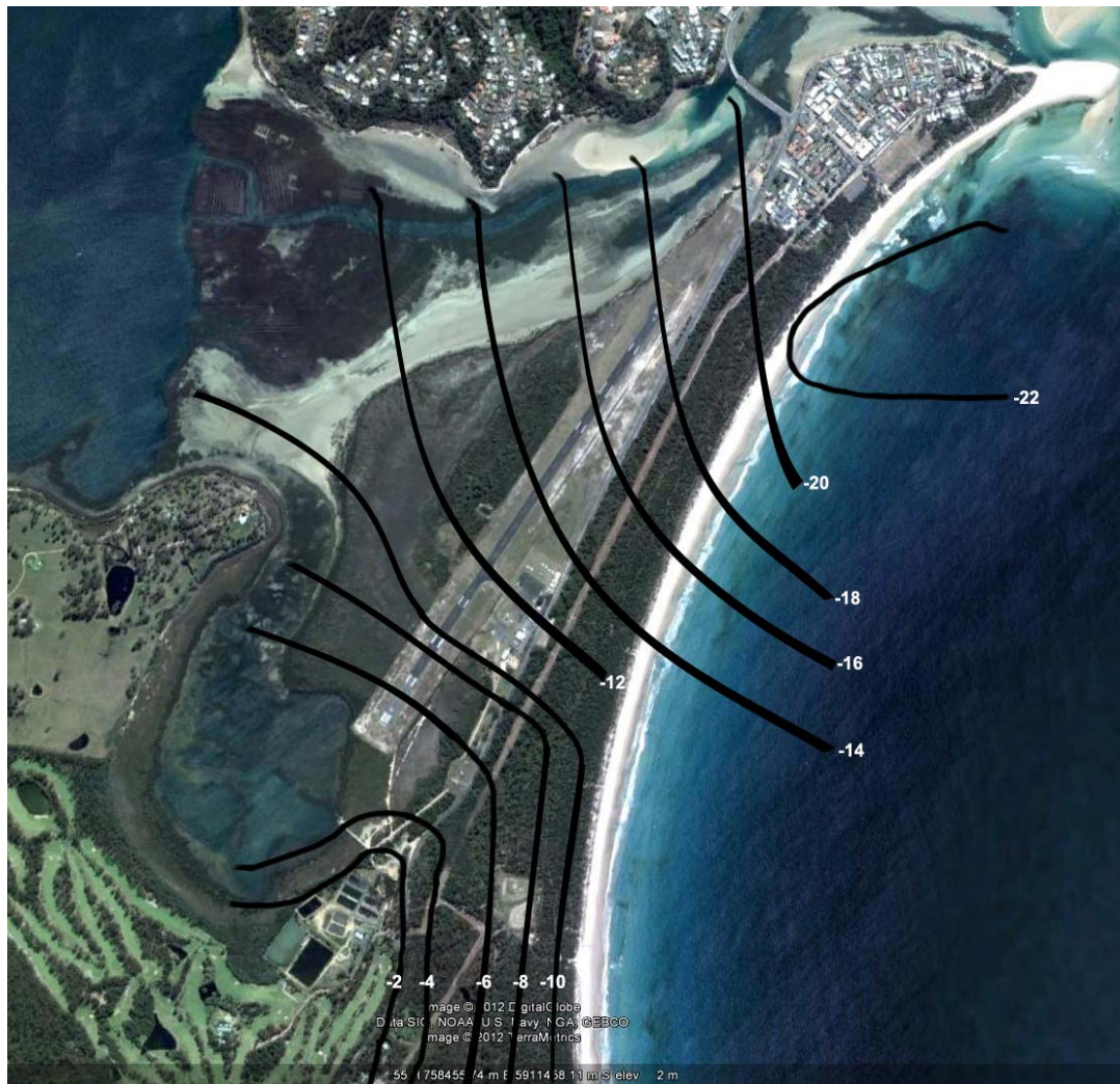
Figure 8.1: Interpreted Base of Shallow Aquifer
