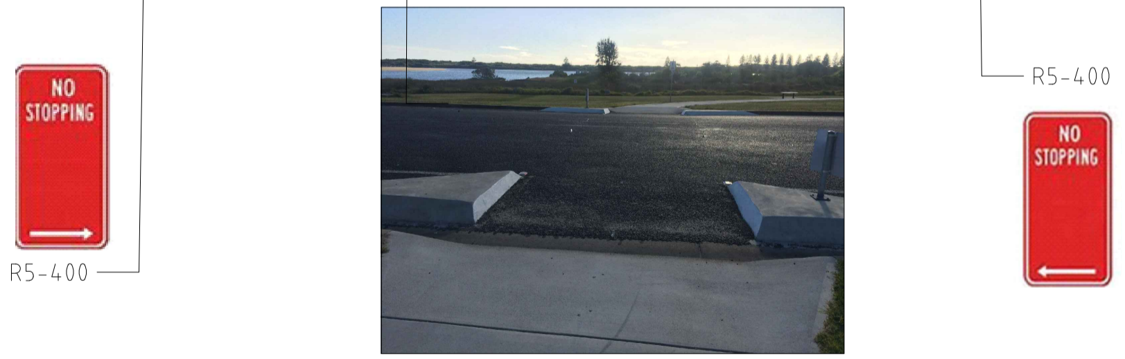
PEDESTRIAN CROSSING LAMONT STREET BERMAGUI CROSSING IN ACCORDANCE WITH RMS TECHNICAL DRAWING T000711 BLISTERS IN ACCORDANCE WITH RMS TECHNICAL DRAWING T000962
