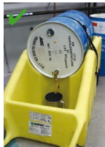
Above left: Hoses, pipes and taps can rupture or fail for a variety of reasons. This activity poses a high risk of water pollution because there is no method of secondary containment. Above right: Decanting smaller containers requires planning and management.
