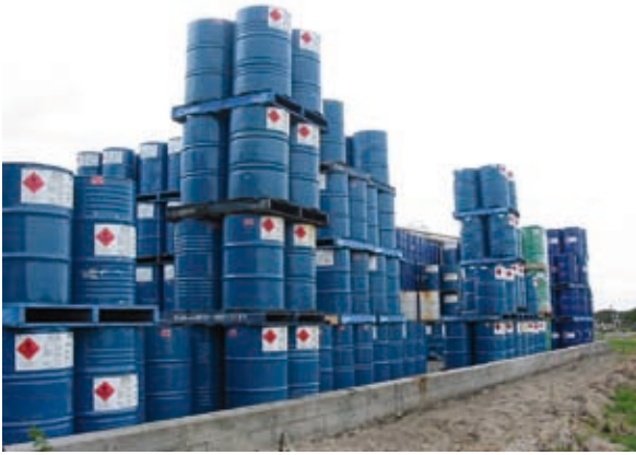
Above: The risk of water pollution or soil contamination from this storage area is high. Leaks from upper drums may not be contained and toppling is likely.
