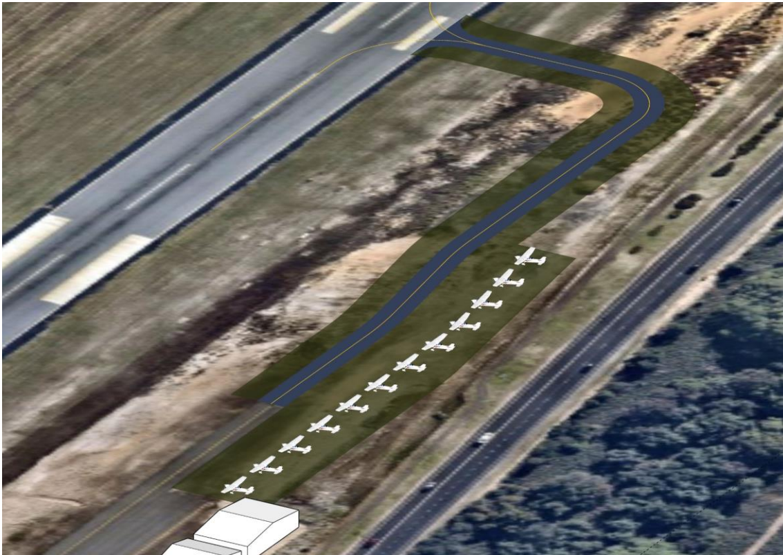
Figure 13: Itinerant Aircraft Parking and Taxiway F Extension
