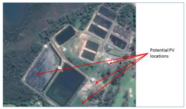
Figure 3: possible solar PV locations at Merimbula STP
